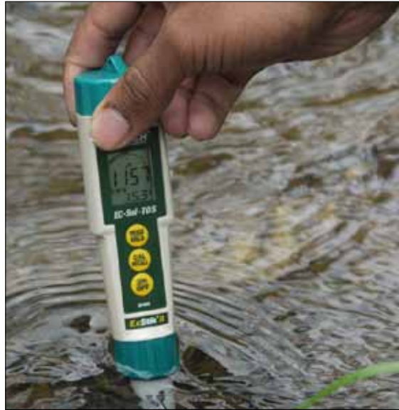
A meter placed in a stream below a mountaintop removal valley fill reveals the stream's high conductivity levels.
