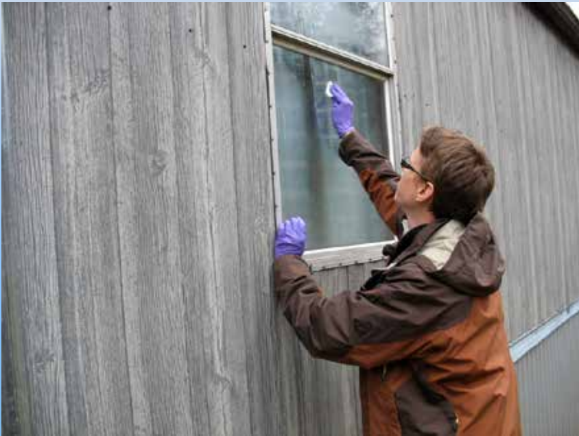
Geochemical window wipes
