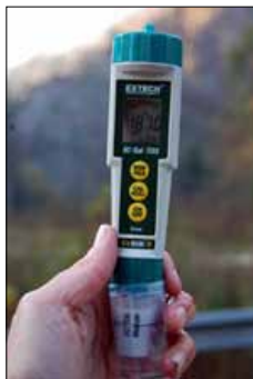
A conductivity meter, for monitoring streams.
