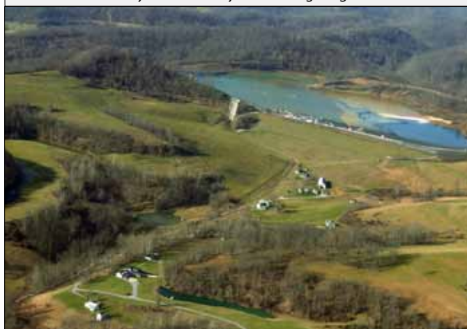
Above: At left, note the failed area of the embankment at CONSOL's Harrison County, W.Va. coal sludge dam. Below: Dwellings near the sludge impoundment. Flyover courtesy SouthWings.org.
